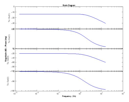
Just as with the umat and uss classes, the Uncertainty property is an atomlist object, acting as a gateway to the uncertain atoms. Direct access to the atoms is facilitated through Uncertainty. Change the nominal value of the uncertain element named 'p1' within sysg to 14, and replot the Bode plot of the (new) nominal system.
