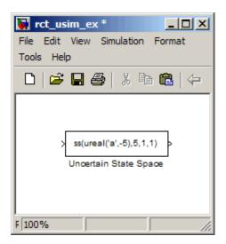
**2** In the Simulink model, double-click the Uncertain State Space block to open the Function Block Parameters: Uncertain State Space dialog box, as shown in the following figure.
