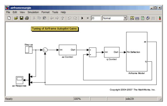
**2** Define a margin analysis point at the output of the Airframe Model block by typing:
