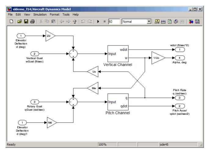
3 Specify uncertain variables for the gain blocks Zd and Mw in the Aircraft Dynamics Model subsystem.
