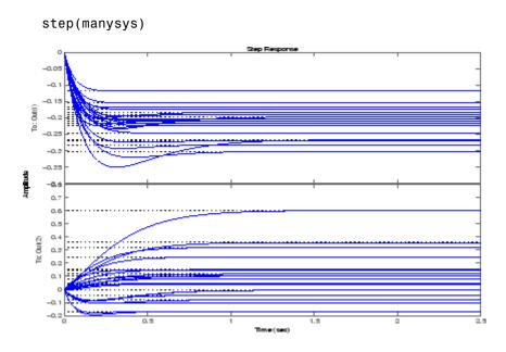
The command step can be called directly on a uss object. The default behavior samples the uss object at 20 instances, and plots the step responses of these 20 models, as well as the nominal value.
