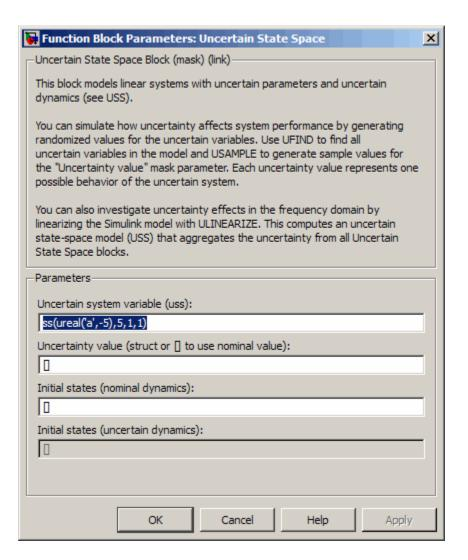
3 Specify an uncertain state-space model in the Uncertain system variable (uss) field. The model must be an uss object or any other model that can be converted to uss, such as umat, ureal and ultidyn. The model depends on a set of uncertain variables (ureal or ultidyn) and you can specify the model as one of the following:
